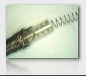
Contributing to this accident was the Federal Aviation Administration's failure to require the installation of nonconductive oxygen hoses after the safety issue concerning conductive hoses was initially identified by Boeing.
